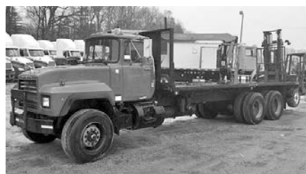
'00 Mack RD690 Moffett truck, 18F, 38R, Mack E7 300 hp, camelback susp., 7 spd., 260" WB, 23' steel flatbed, $14,500.
