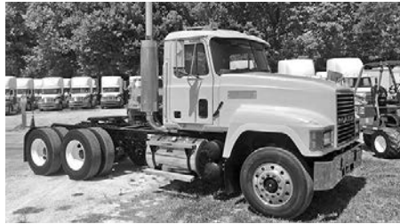
'97 Mack CH613 tdm. day cab, Mack E7, 350 hp, 470,000 original miles, camelback susp., 38R, 192" WB, Mack 9 spd., alum. whls. on frt., clean, local truck, $19,500.
