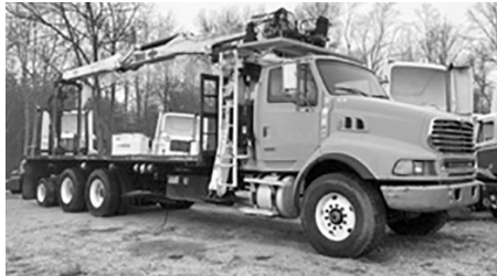
'06 Sterling LT9513 tri-axle boom truck, MBE460 450 hp, Allison 4560 auto., 24.5' flatbed, 226,000 miles, Jake, TufTrac spg. susp., 20F, 46R, dbl. frame, full locking rears, $45,000.
