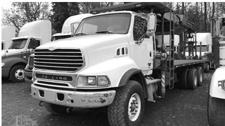
'07 Sterling LT9513, MBE460, 10 spd., 20F, 46R, dbl. frame, full locking rears, 350,000 miles, $38,500.
