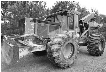
'08 Deere 648H D/A, w/torque convertor, winch, 10,015 hrs., reman eng., 30.5x32, $75,000.
