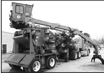
'05 Morbark 23WCL Chiparvestor, Cat 3412, 860 hp, log ldr., A/C cab, rem. control, 3-knife 75" chipper, separator, clean & painted, $127,500.
