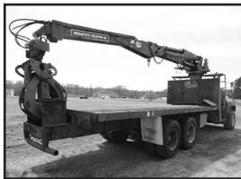
'94 Mack DM 690 chassis, 22' steel bed, Prentice Telstik 33' extend boom, log grapple, truck runs good, not highway approved, $20,000.
