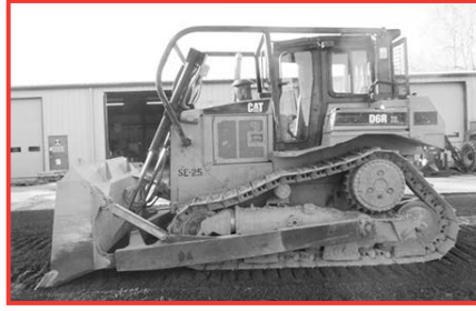
'02 Cat D6RXL dozer, 190 hp, 6-cyl., encl. cab, A/C, pwr. shift trans., diff. steering, semi-U 10'6" pwr. tilt blade, sweeps, 24" single grouser pads, draw bar, stk. #8200, $76,900.
