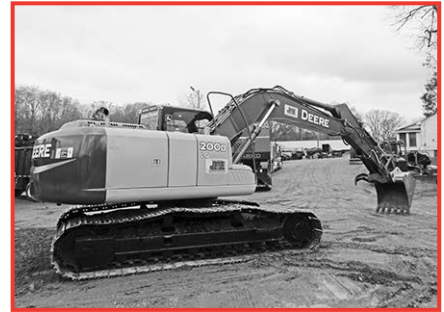
'11 Deere 200 DLC excavator, 4353 hrs., 6068H eng., 159 hp, 32" tri- ple grousers, 46" bucket, hyd. thumb, Stock #7336, Price: $96,000.
