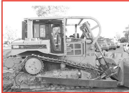
'07 Cat D6RXL dozer, 190 hp, 6-cyl., encl. cab, A/C, pwr. shift trans., diff. steering, semi-U blade single tilt, Paccar winch, sweeps, 24" single grousers, system one U/C, stk. #8201, $99,000.
