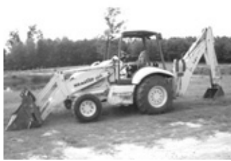
'00 Komatsu WB140-2, 4x4, ldr. backhoe, OROPS, 4-in-1 ldr. bucket, std. stick, 24" bucket, $22,500.
