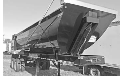
'22 Clement frame-type construction/ demo trlr., 28' long, 2-way gate, 1/4 AR 450 steel body, great all around trlr., call for price.
